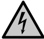
Electrical shock hazard
